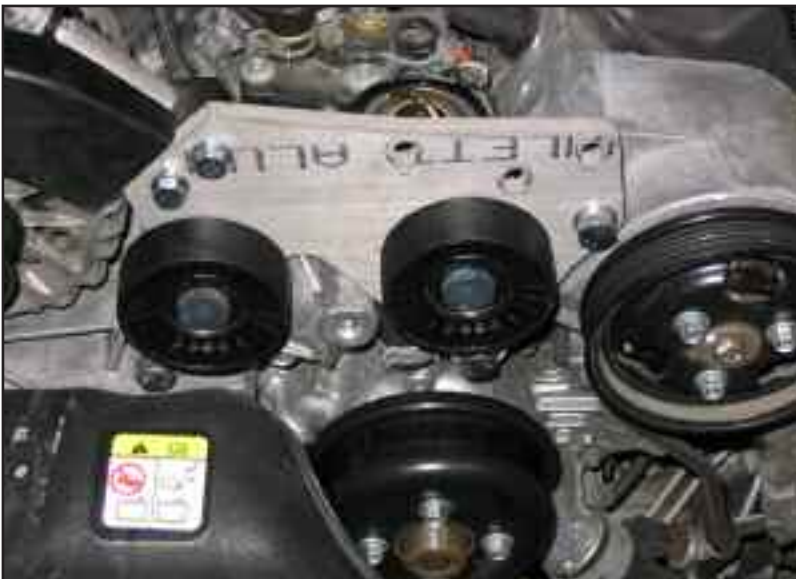
Figure DE install idler pulleys
