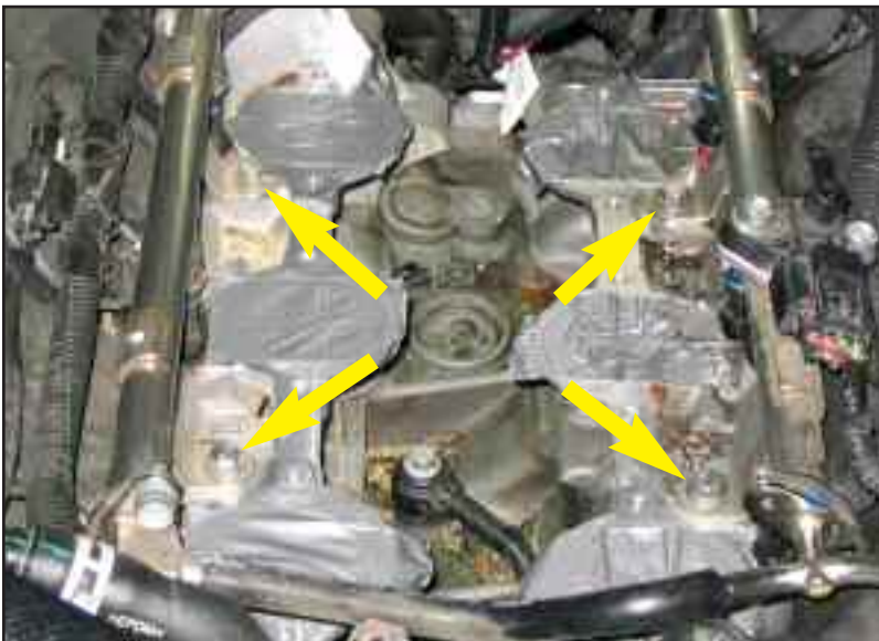
Figure IC fuel rail bolts
