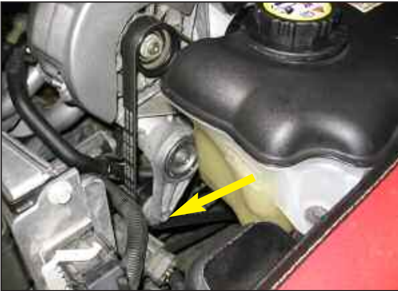
Figure U Remove drivebelt
