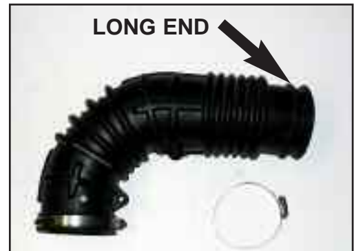
Figure ABO cut clamp retainer from this end
