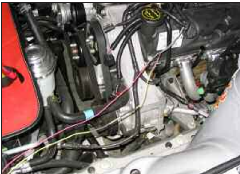
Figure HL cut ACT wires
