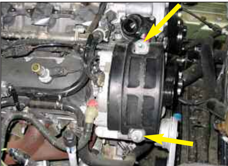
Figure V remove alternator cover
