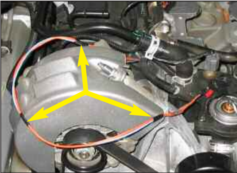
Figure HO tape Throttle Actuator wires
