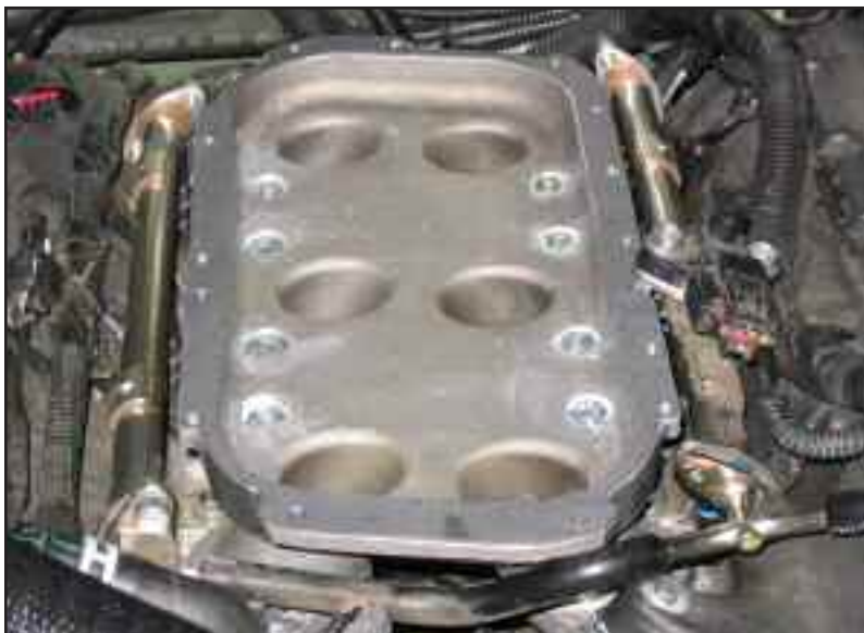
Figure AF install discharge manifold
