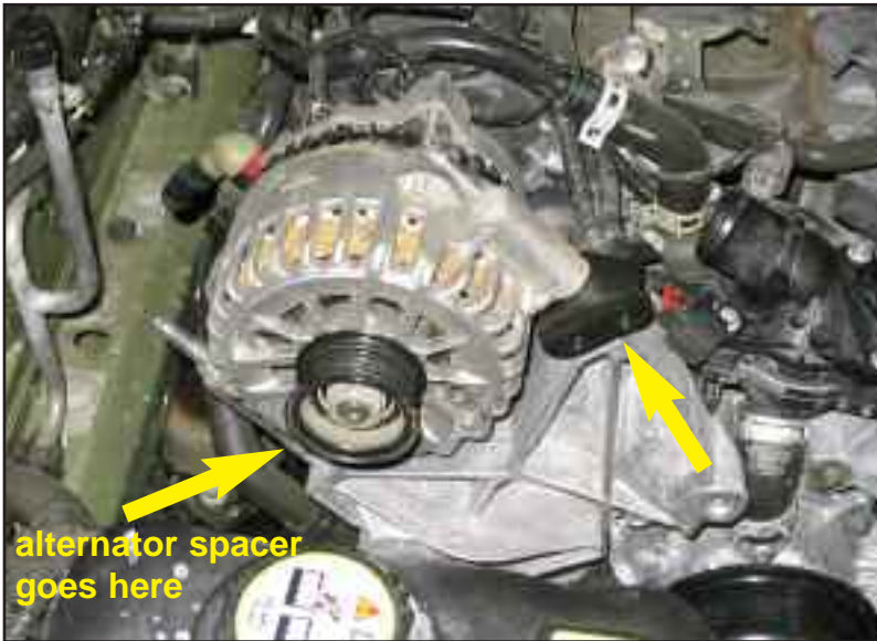
Figure DA install alternator spacer and bracket
