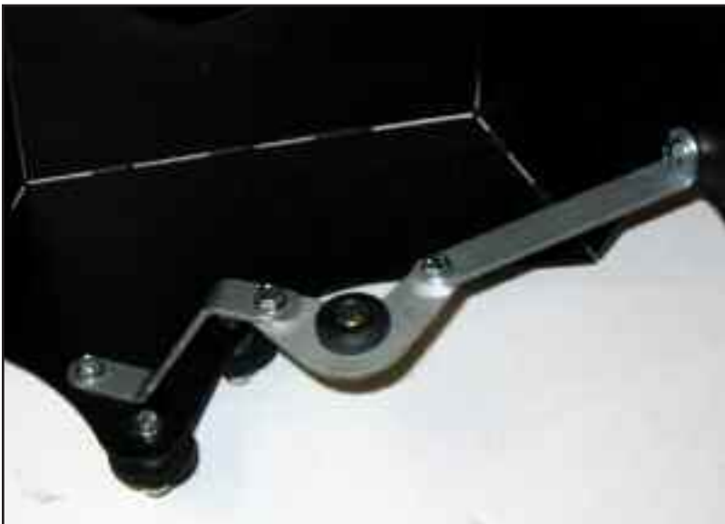
Figure ABI install airbox retainer
