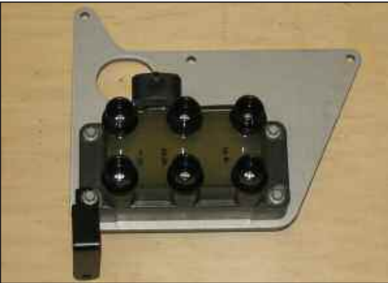
Figure AC coil and bracket
