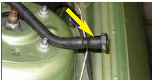
Figure AR remove hose connector
