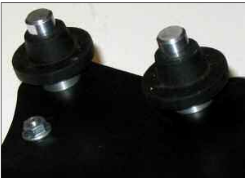
Figure ABJ install airbox insulators
