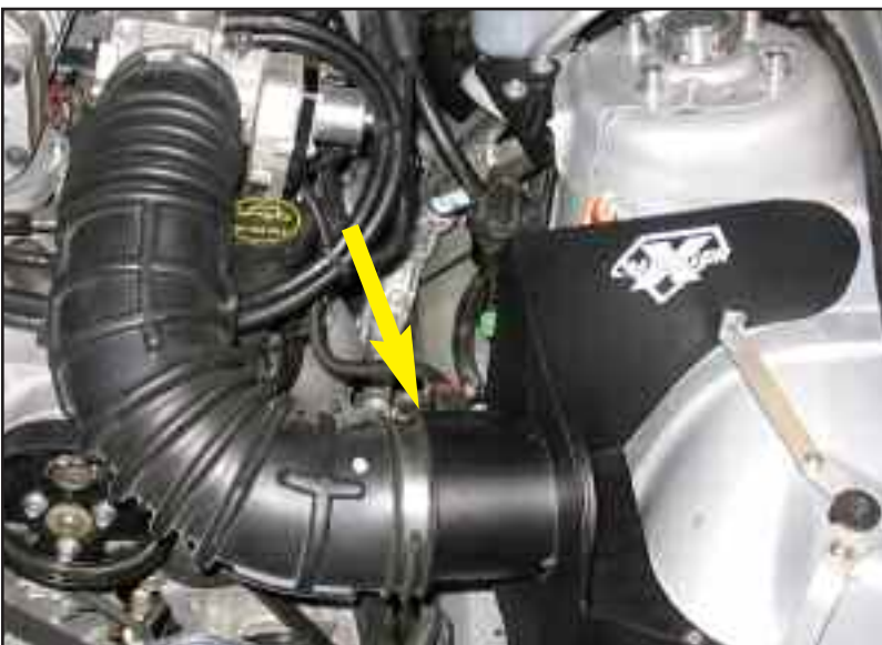
Figure ABP install inlet hose
