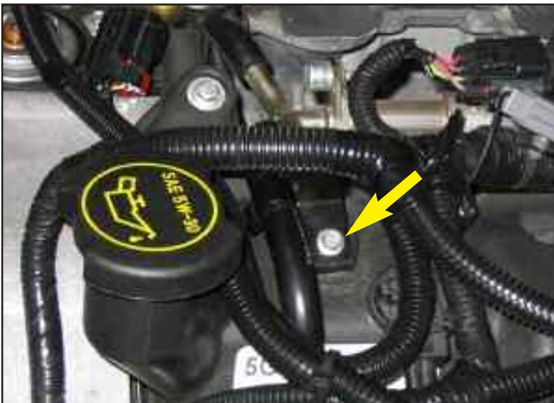
Figure IA remove fuel line bracket
