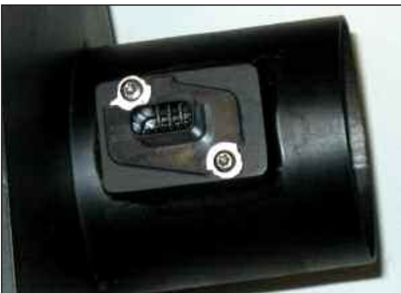
Figure ABL install MAF sensor
