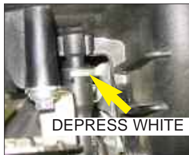
Figure O-2 vapor hose connector
