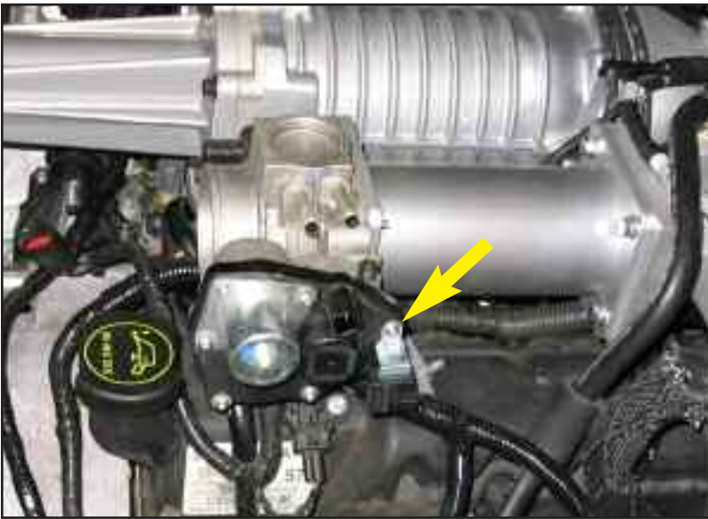
Figure AU coil resistor
