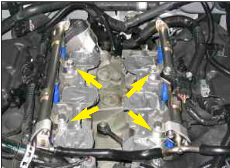
Figure II install fuel rails and spacers
