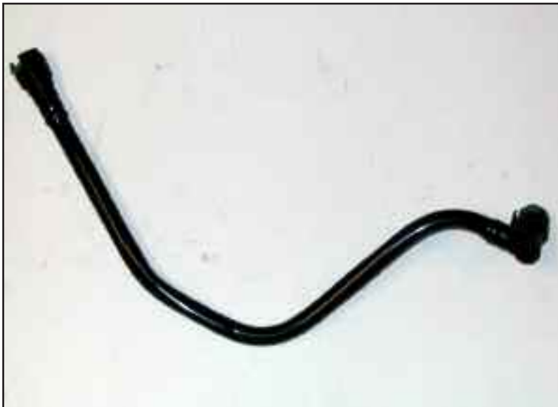
Figure BC complete new PCV tube
