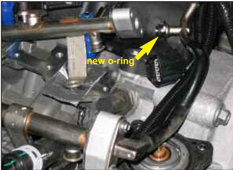
Figure IH install fuel rail extensions
