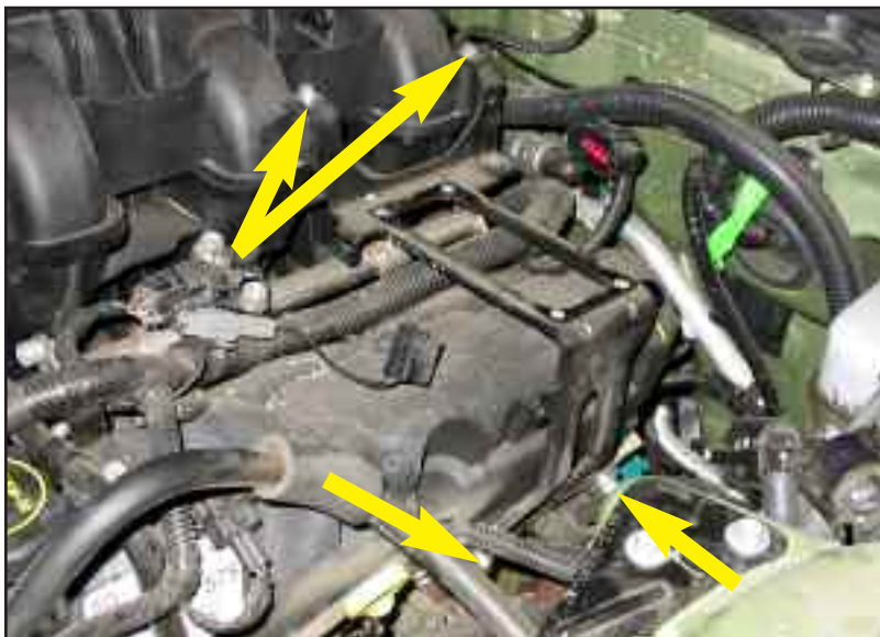
Figure N remove coil bracket
