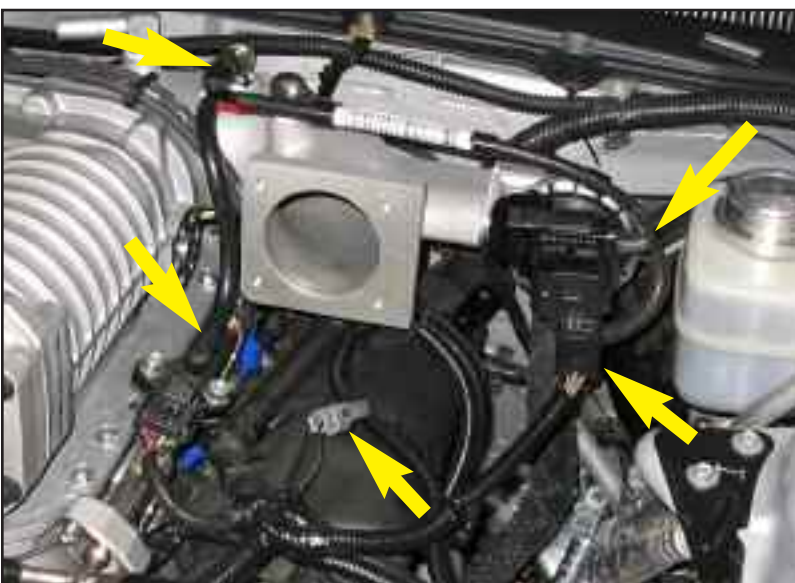
Figure AQ vacuum source tube
