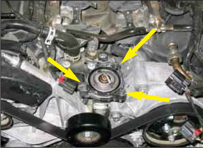
Figure T remove thermostat cover dowels
