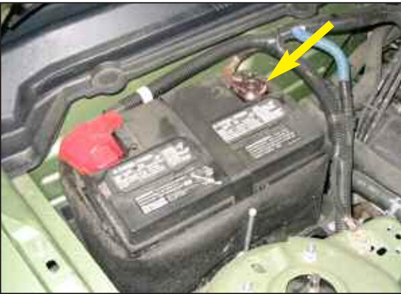
Figure B disconnect battery
