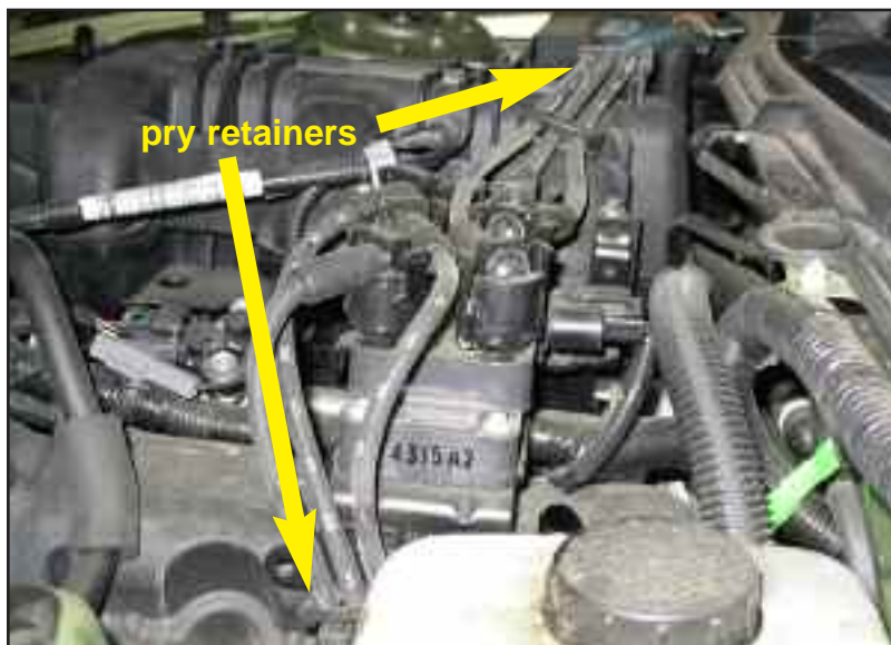
Figure L remove plug wires
