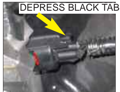
Figure IE-1 injector connector
