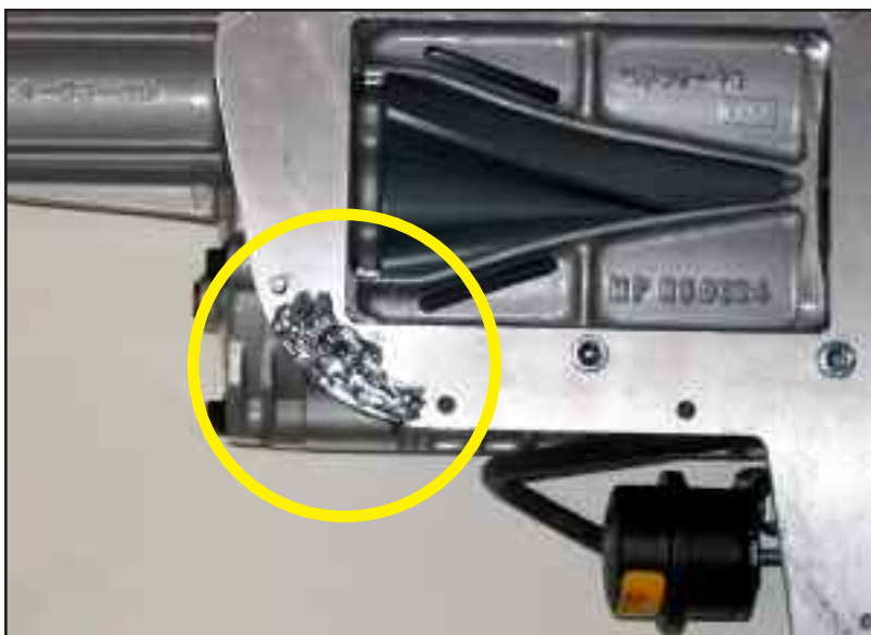
Figure AH apply sealer to discharge lid
