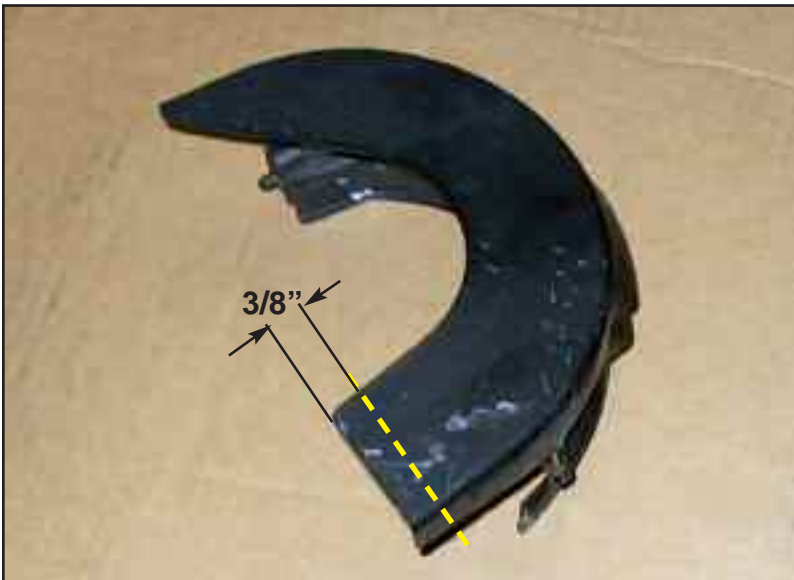
Figure W modify alternator cover
