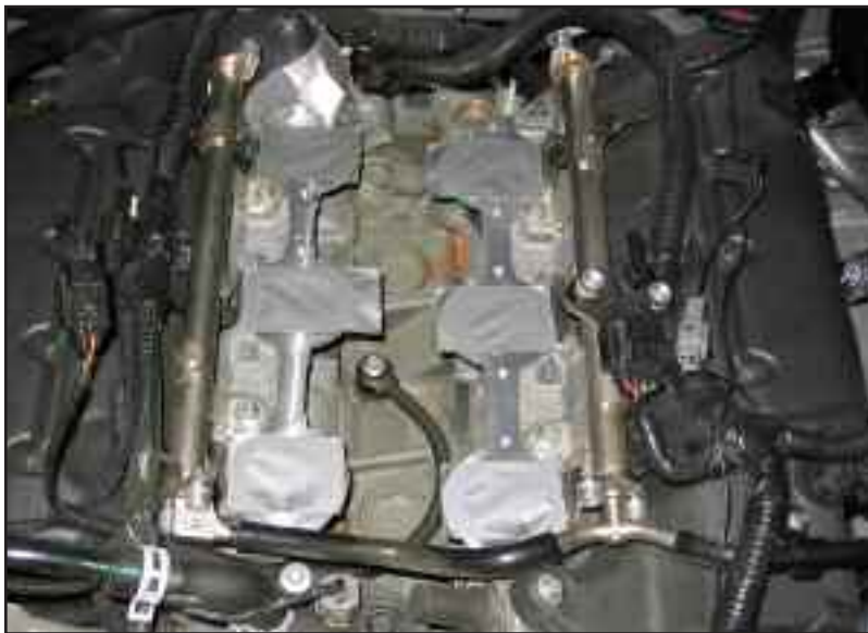
Figure R tape intake ports
