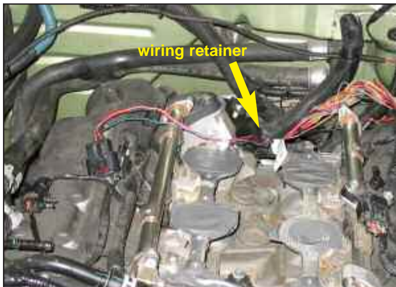
Figure HC pull coil wires from harness
