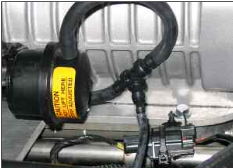
Figure ABT connect boost gauge
