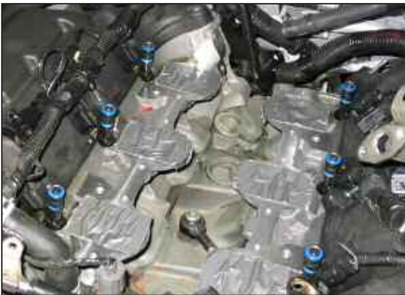
Figure IE injector orientation
