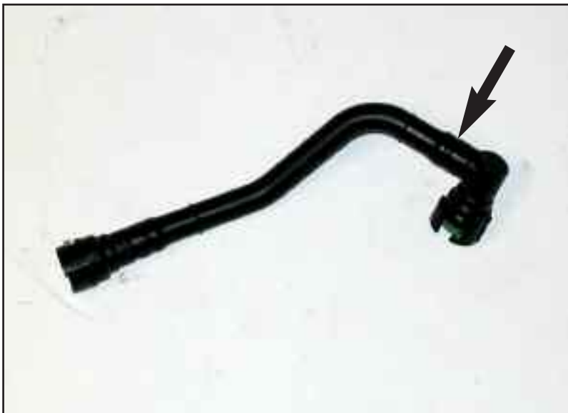
Figure BA remove PCV valve fitting
