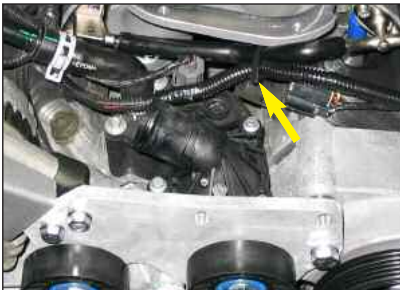
Figure AA install thermostat cover
