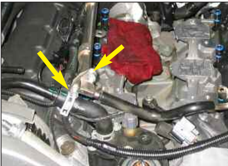
Figure ID disconnect right fuel rail
