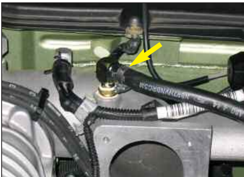
Figure AR vapor hose installed
