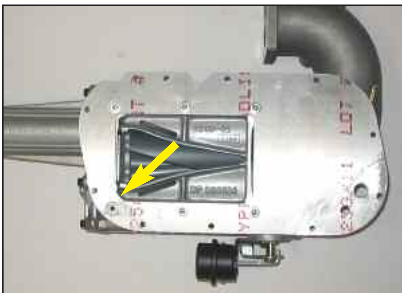
Figure SF install discharge manifold lid
