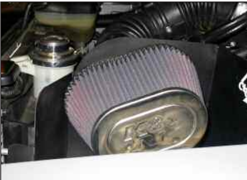
Figure ABR install air filter
