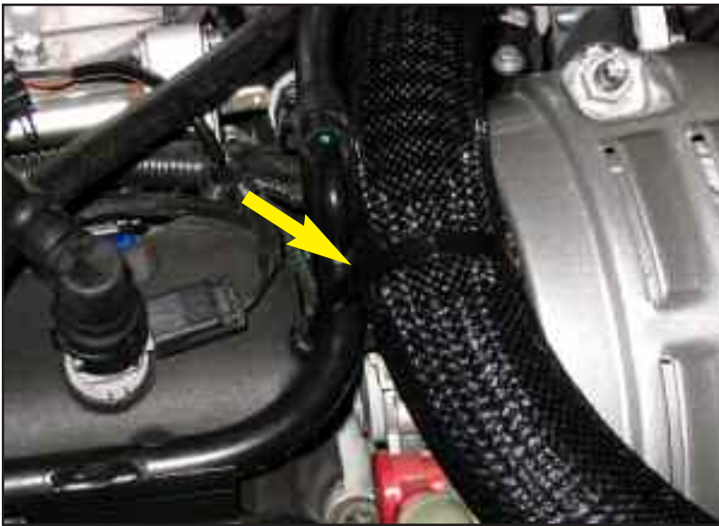
Figure AX radiator hose tiewrap
