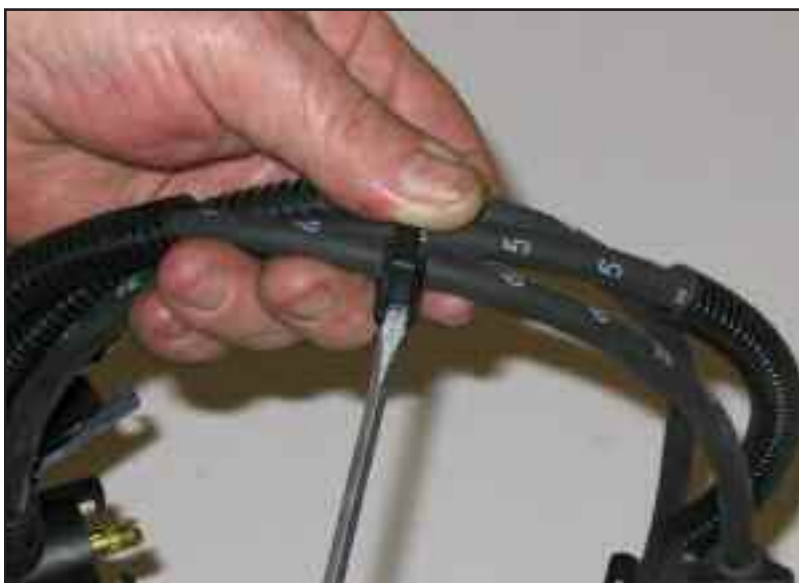
Figure AJ remove plug wire retainers
