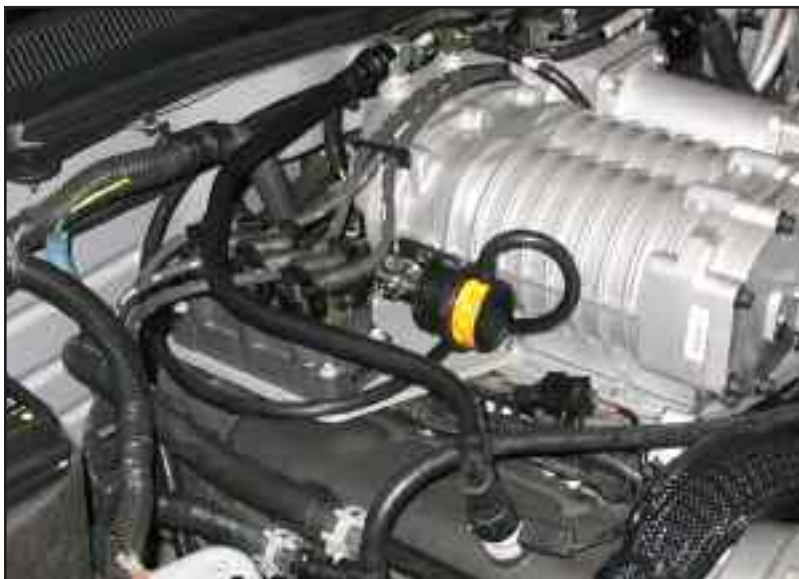
Figure ABA PCV tube installed
