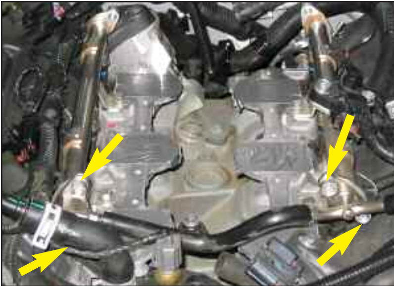
Figure IB loosen fuel crossover bolts
