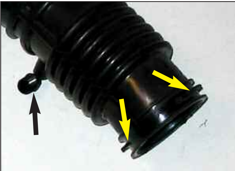
Figure ABN cut off hose clamp retainers
