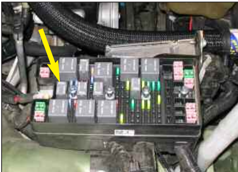
Figure A remove fuel pump relay
