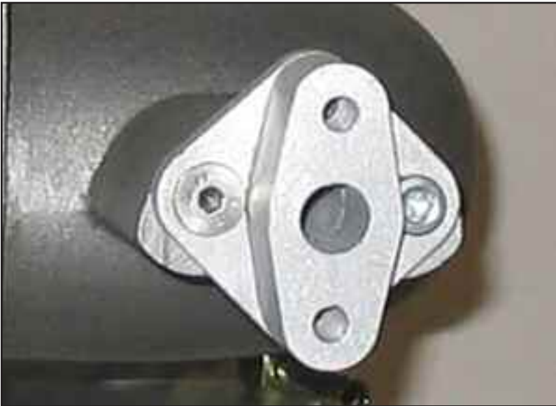
Figure SG install EGR adapter
