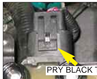
Figure M-1 coil connector
