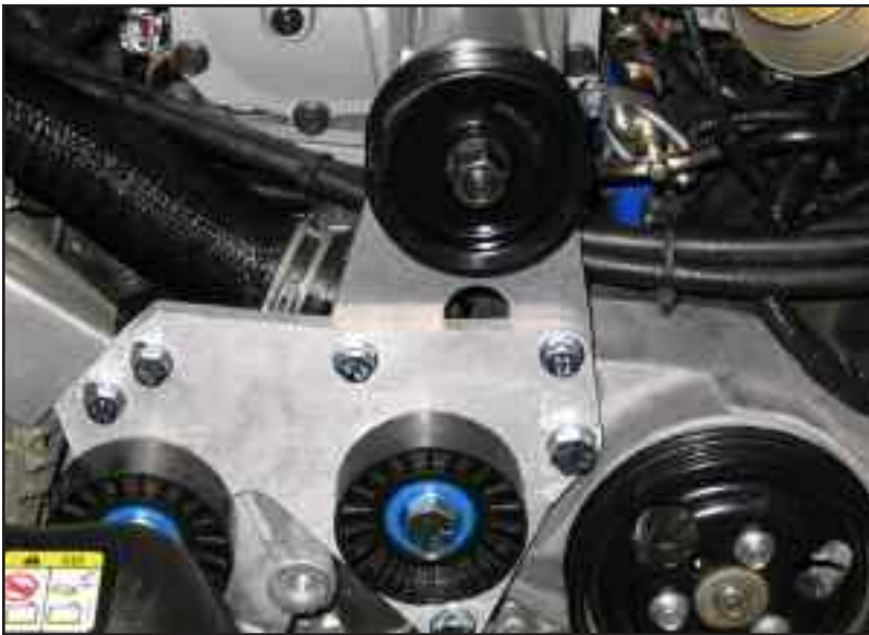
Figure AY install nose support
