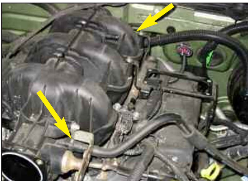
Figure O remove vapor and booster hoses
