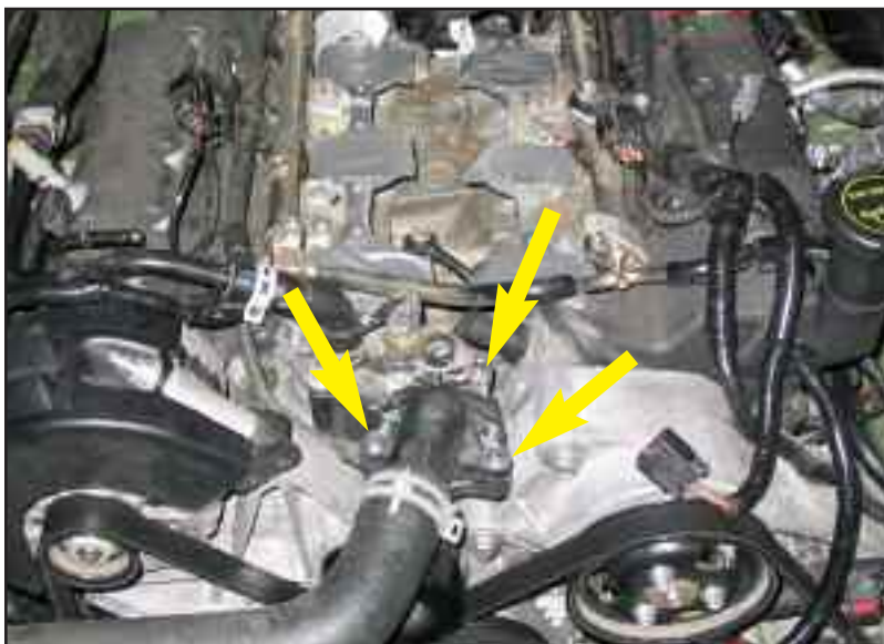
Figure S remove thermostat cover and upper rad hose
