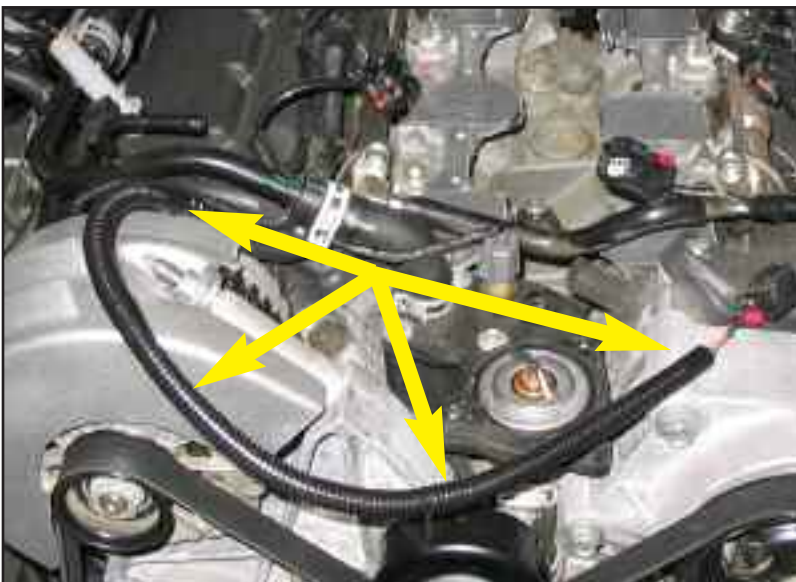
Figure HP install Throttle Actuator wire armour
