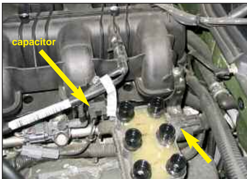
Figure M disconnect coil
